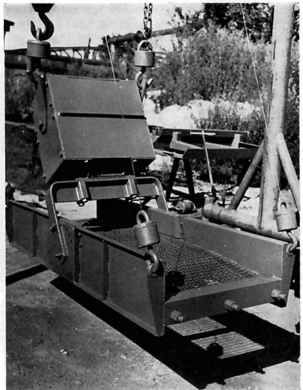
Fig. 10: Vibrating screen electromatic driven
