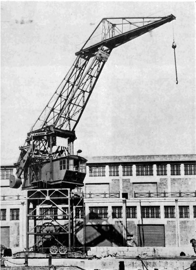
Fig. 1: Gantry luffing swing crane, 5 tons capacity and 15,4 meters maximum outreach
