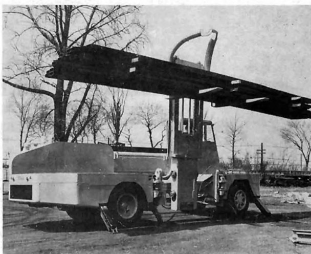
Fig. 9: Side-loading fork-lift transporter for stacking and transporting long beams
