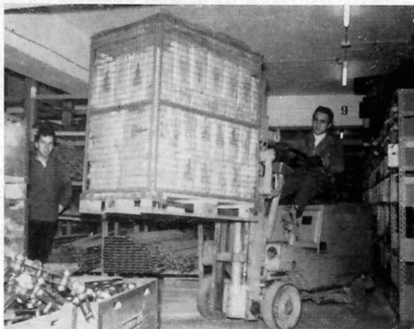
Fig. 8: Fork truck with collapsible wire mesh pallet
