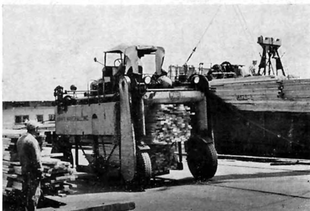
Fig. 10: Straddle carrier for the transport of long loads
