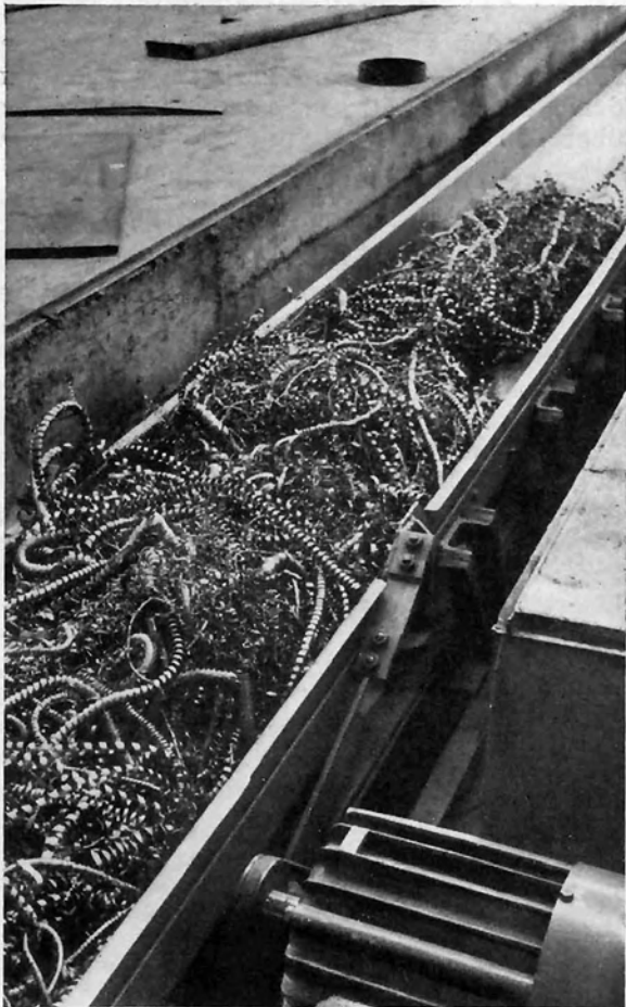
Transport of shavings with vibrating conveyors in a modern machine manufacturing plant
