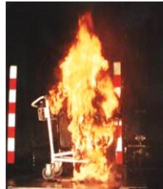
1.2MW peak heat release rate
